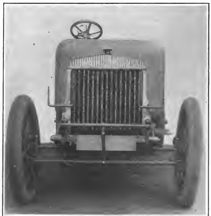
FRONT OF DAIMLER 28-36-HORSEPOWER CHASSIS, SHOWING RADIATOR.
